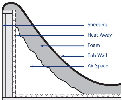
Radiant Barrier (Hotter water at a lower thermostat setting.)
