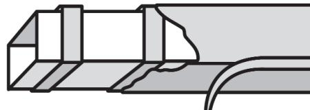
R-6 (with airspace) dramatically reduces duct leakage.
